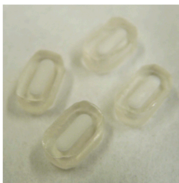
Figure 1. Photograph (top view) of four oblong pre-F-containing core-shell implants (approximately 5 \times 9\text{ mm} ). The core (approximately 25 mg) consisted of a physical mixture of freeze-dried pre-F-containing powder (24 wt %) and mannitol (76 wt %). The shell consisted of PLGA.
