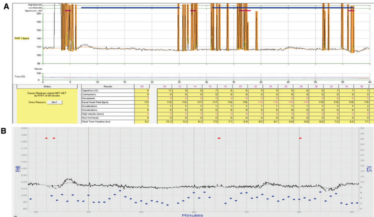
Figure 3: Cardiotocography tracing by FetalCare in panel A, and by STVcalc in panel B. (A) FetalCare STV of 6.2 ms over 60 min. Very flat pattern with spikes. Note the very high early STV values in the bottom row of the yellow table below the graph. (B) STVcalc filtered out the signal loss in the beginning and the spikes (small horizontal bars above graph) and calculated STV of 3.4 ms. Case description: Para 0, referred at 29 + 5 weeks after eclampsia, stabilized with magnesium and antihypertensive treatment. Corticosteroids given. Current CTG at 29 + 6 weeks. Caesarean section for maternal and fetal condition 1 day later: female, 920 g, no severe neonatal complications.
