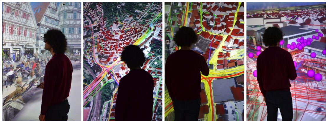
Figure 4. Stereoscopic visualization in the CAVE: a) Visualization of the current situation with the help of point clouds in scale 1:1, walking-mode; b) Visualization of space syntax NACH analysis in 3D-VR linked to data of particulate matter and airflow analysis in big scale and flyby-mode; c) Overlay of space syntax analysis and movement patterns; d) Movement patterns combined with other VGI data collected with the mobile application.
