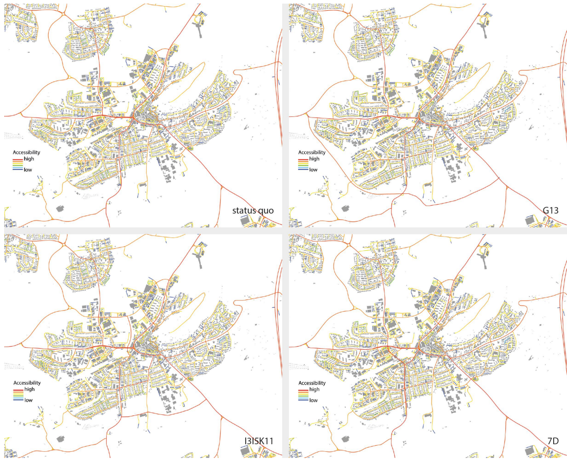
Figure 3. NACH analysis of three traffic planning scenarios and the current situation in 2D.
