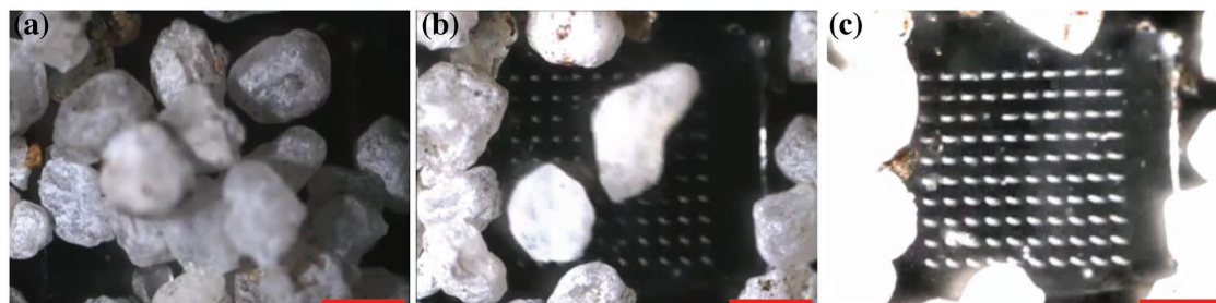
Figure 5. Removal of real sand grains by magnetic artificial cilia. Snapshots from one recorded experiment after the MAC operate for a) 0 s (because the sand grains have a larger size than the cilia pitch, they all settle on top of the cilia tips initially), b) 16 s, and c) 30 s, showing that all sand grains are gradually removed from the ciliated area. In this experiment, the MAC performed the ITC motion, and the rotating speed was initially 0.1 Hz and was then suddenly increased to 40 Hz. All scale bars are 1 mm. See also Video S8 (Supporting Information).
