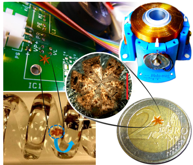
Fig. 1 Top Left : Image of a soft untethered gripper on a printed circuit board. Top Right : The electromagnetic setup consisting of six orthogonally-oriented electromagnetic coils. The electromagnetic coils have a cutoff frequency of 70 Hz and a maximum current rating of 1 A. The system generates a maximum magnetic field and magnetic field gradient of 15 mT and 60 mT/m, respectively. Center : Image of the closed gripper. Bottom Left : Video snapshot images of the gripper navigating through a tube with an inner diameter of 3.2 mm, a size smaller than most of the major vessels in the human body. Bottom Right : Image of the gripper on a 2€ coin. The scale bar is 0.4 mm
