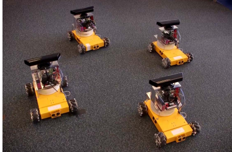
Figure 1.3: Mobile robots with Mecanum wheels in DTPA Lap, University of Groningen. With onboard sensors and controllers, each robot can acquire position information of the others and adjust the speed and rotation accordingly to achieve a certain formation.
