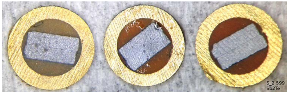
Figure 2.12: Cut disks out of the brass tube. The epoxy used in this case is Gatan G1, which gets an amber color after the cure. As can be seen, the specimen on the left is not cured, while the two on the right are cured at progressively higher temperatures.
