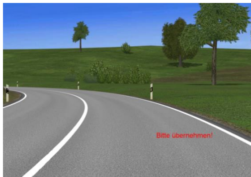
Figure 2. Screenshot of the driving scenario in the moment of take-over request in the curve ("Please take over!")
