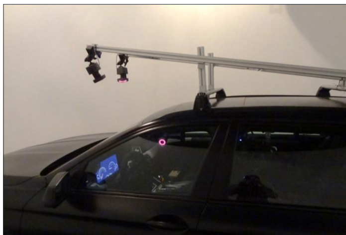
Figure 3. Motion tracking systems implemented in the mock-up vehicle.
