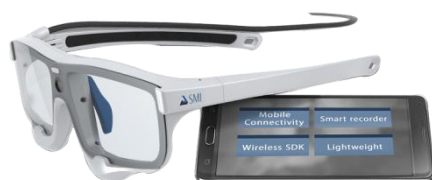
Figure 3. SMI eye tracking glasses 2 with recording unit
