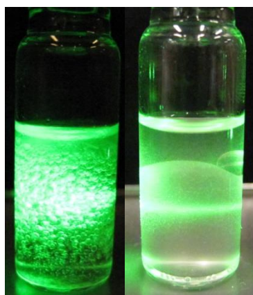
Figure 5 A mixture of styrene and water shows the extent of scattering of light (532 nm) from a Raman probe, held externally to the vial, during rapid stirring and after standing to allow phase separation (left: vigorously stirred, right: after 10 min standing).
