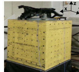
Figure 1: A rear sub-frame of a car mounted on CUBE shaker
