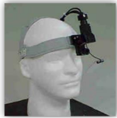
Figure 1. The ASL Head-Mounted HS-H6 Eye Tracking System.
