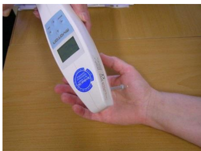
Figure 6, 7. Myometer for muscles stiffness measurements
