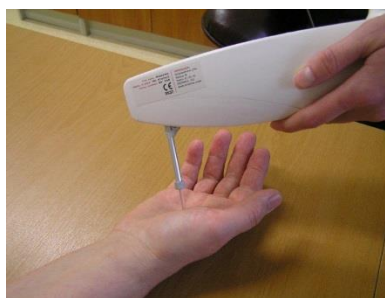
Figure 6, 7. Myometer for muscles stiffness measurements
