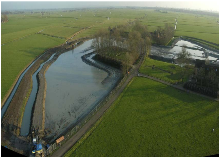
Figure 3.5: Several terps have been (partially) refilled with dredging material. This oblique aerial photo shows the refill of Wierum, with the original terp remainder in the centre. (Photo: H. Breedland, Province of Groningen)
