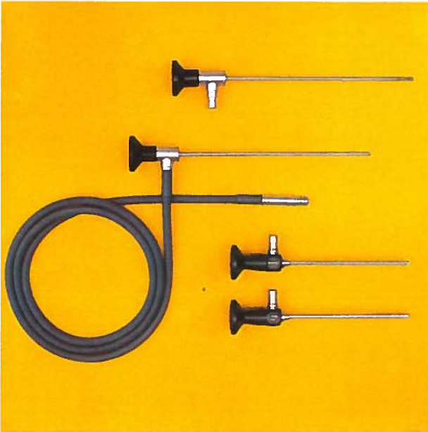
Picture 4. Optics for nasendoscopy. Above, 160° and 100° (photo) Lumina optics, Ø 4 mm (Wolf nomenclature). Below, 30° and 70° Hopkins optics, Ø 4 mm (Storz nomenclature).
