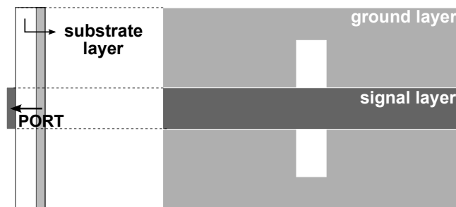
Figure 1: Elementary section of a defective ground plane resonator filter. Left: cross-section. Right: top-view.
