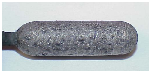
Figure 4.66. Specimen # 40 after first \text{CrCl}_3 -50Cr (wt.%) layer has been LIC applied. Almost a 100% coating coverage has been obtained.
