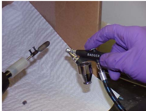
Figure 3.10. Spray painting of cylindrical sample using a Badger™ air-spraying gun.
