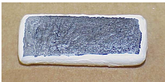
Figure 4.54. Specimen #261 prepared for weight loss testing, coating consisted of Si-10SiC-10CrCl 3 -30HfC (wt.%) and SILBOND TM overcoat layer.
