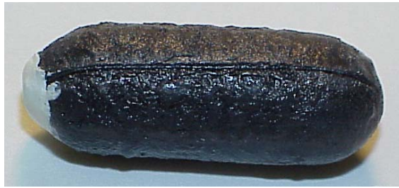
Figure 4.60. Specimen # C2 as coated and prepared for weight loss testing.
