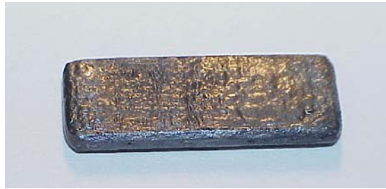
Figure 4.55. Specimen #270, after being laser fusion coated at both sides.
