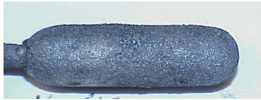
Figure 4.67. Specimen # 40 after the second Si-25Cr-5CrCl 3 -5C (wt.%) layer has been laser fused. A smooth coating has been obtained all over the surface.
