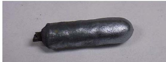
Figure 4.61. Specimen #17 after the LIC coating process. Surface is covered completely and appears smooth, homogenous and silver in color.
