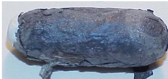
Figure 4.136. Specimen # C2 after weight loss test at 1000 °C in flowing air.
