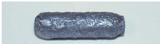
Figure 4.63. Specimen # 24 as LIC processed, surface is covered completely but lumps are spread over the coating. Stem has been removed.
