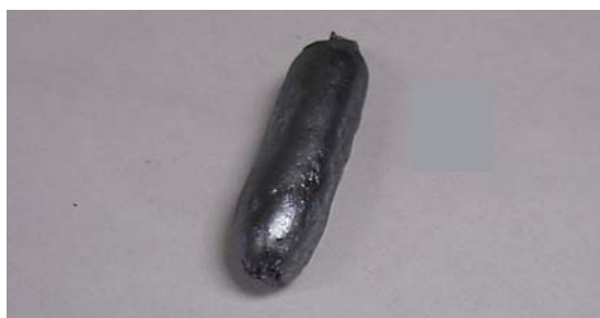
Figure 4.62. Specimen #18 after the LIC coating process. Surface is covered completely and appears smooth and uniform.
