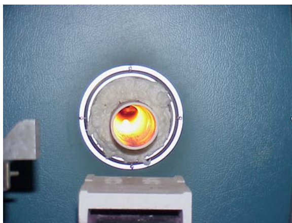
Figure 3.14. Horizontal furnace operating at 1000 °C under direct air with a coated cylindrical sample being weighted loss tested.
