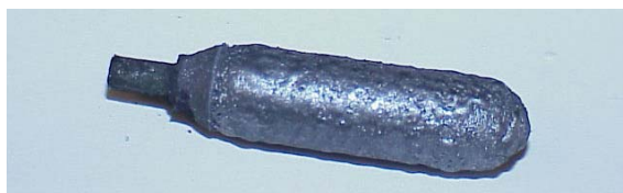
Figure 4.65. Specimen # 32 as LIC processed, surface is covered totally and appears smooth.
