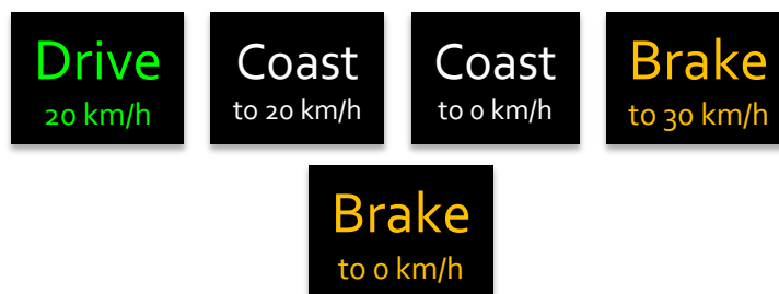
Figure 1. Driving recommendations as shown in the HMI. The drive recommendation was depicted in green, coast recommendations in white and brake recommendation in amber.
