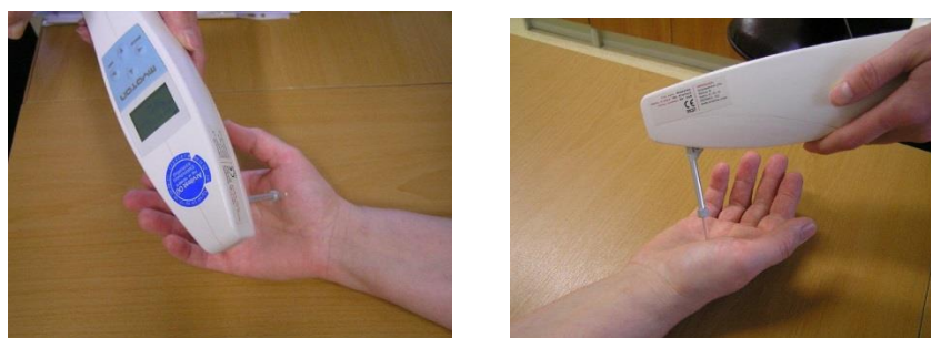
Figure 6, 7. Myometer for muscles stiffness measurements
