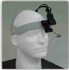
Figure 1. The ASL Head-Mounted HS-H6 Eye Tracking System.
