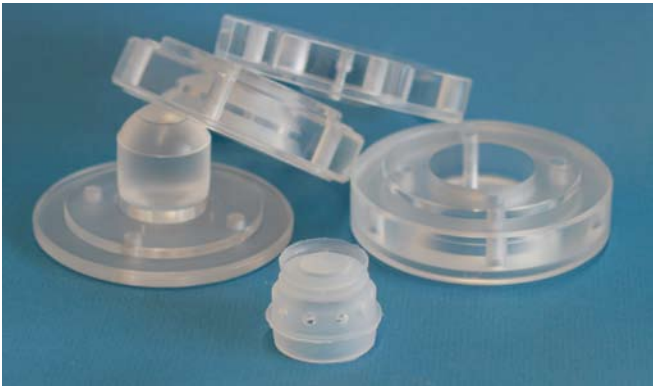
Figure 12. The iValve v2 (foreground) in the shape it is molded in, before it is flipped inside-out. The mold is in the background.
