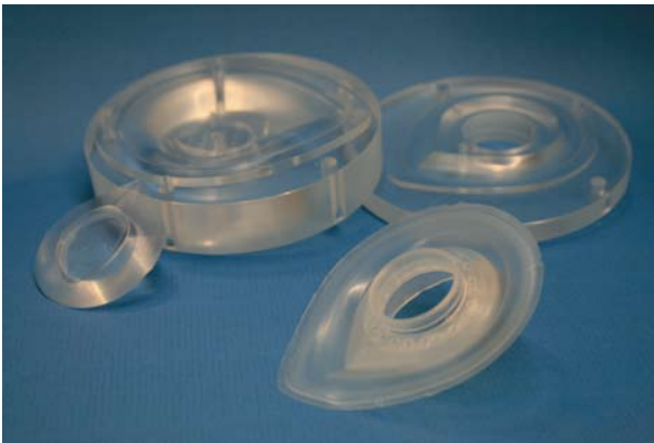
Figure 8. The drop-shaped iPatch v2 (foreground) and its mold (background).
