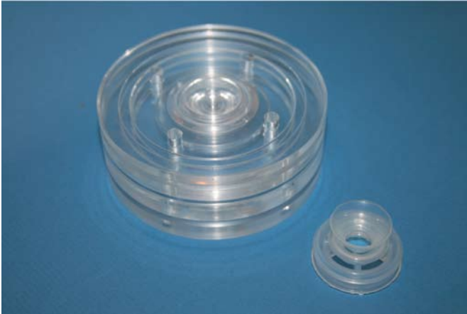
Figure 10. A silicone rubber product (iValve v1, capseat part ) with a typical mold as used for the creation of all the rubber products in this thesis (background).
