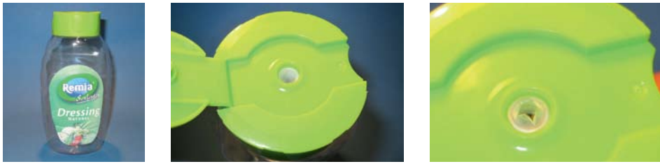
Figure 1. Weener-Ibérica (Weener Plastic Ibérica, S.L., Spain) non-drip valve as can be found in sauce or shampoo dispenser caps (left and middle): when the bottle is squeezed, the little valve (right) moves forward and then allows the cross shaped slits to open, when the pressure drops the cross closes and the little dome retracts, shedding the remaining droplets: the valve cleans itself.
