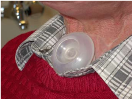
Figure 8. iValve v1 on a patient, attached by means of an Atos Optiderm adhesive patch.
