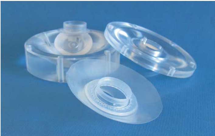
Figure 6. The iPatch v1 (foreground) is molded in a three part PMMA mold (background). The connector used in the iPatch is perforated around the perimeter (visible in the iPatch) and inserted into the mold prior to filling.
