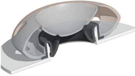
Figure 2. A cross-sectional view of the inhalation valve in closed position (left) and attached to the stoma using an adhesive patch (right).
