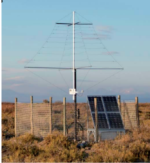
Figure 2.4.1: A photo of an AERA station – The log-periodic dipole antenna (LPDA) can be seen above the horizon. The electronic system where the signal is amplified and digitized is situated below the solar panels to the right of the antenna.
