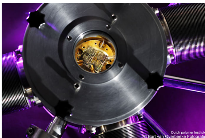
Figure 2.7: Electrical characterization of large-area molecular junctions in a Janis probe station.
