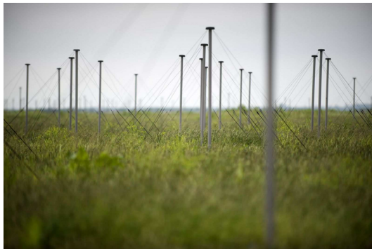
Figure 2.1: An LBA station of LOFAR as an example of a phased-array station, with the simplest antennas, i.e. droopy dipoles (the photo source: http://www.astron.nl/ ). The photo is courtesy of Hans Hordijk.
