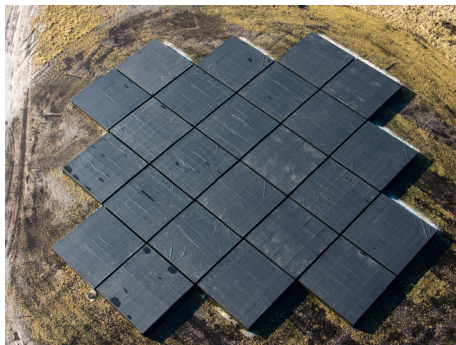
Figure 3.1: Twenty-four-tile HBA station. Each tile is one station element. This is the station configuration for most of LOFAR’s HBA stations, including the LOFAR core (CS302). It is clear that a station like this is highly redundant.
