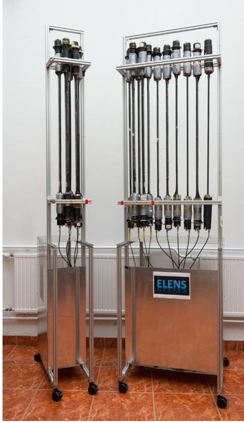
Fig. 4. A photograph of the ELENS array. The PMTs are covered with special mu-metal sheets against possible interference effects caused by the magnetic fields.
