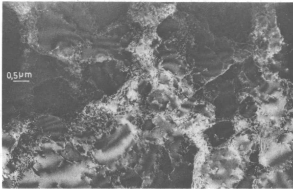
Fig. 10. Cell structure of Al deformed 25% at 77K. Dark field/weak beam image, [100] orientation, g=[002] ; JEM 200 CX.
