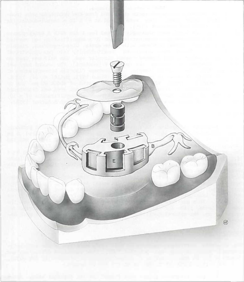
Figure 4.2. The intra-oral device used in the clinical study (S: occlusal part; E: enamel; B: frame body).
