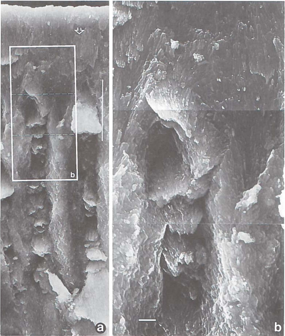
Figure 8.3. SEM-micrographs of control enamel after 4 months demineralization. a. Detail of the demineralized area (the bar is 10 \mu\text{m} ); the acid attack direction is indicated by the arrow. b. Detail of the demineralized area 5-30 \mu\text{m} below the surface (the bar is 1 \mu\text{m} ); note the absence of the globular structures.
