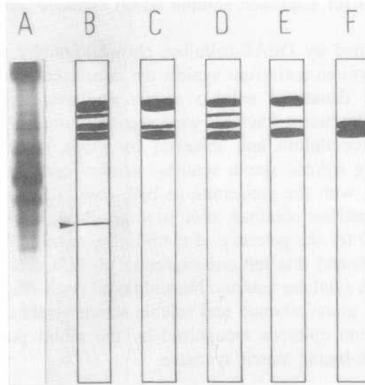
Figure 6: Zymogram patterns of fractions containing soluble starch synthase activity at several stages of the purification procedure. Fractions from Producent potatoes (10 to 20 \mu\text{L} containing 5 mU primed soluble starch synthase activity) were loaded on 8 % PAA gels, and stained for protein (lane A) or primed soluble starch synthase activity (lanes B to F). The protein and soluble starch synthase activity pattern of the ammonium sulphate fraction is shown in lane A and B respectively, and the activity pattern obtained after passage through DEAE-cellulose is shown in lane C. Further purification by aminobutyl-Agarose gives the patterns shown in lane D (retardation) and E (elution with 1 M maltose in buffer). After Superose-12 chromatography the pattern shown in lane F was found.
