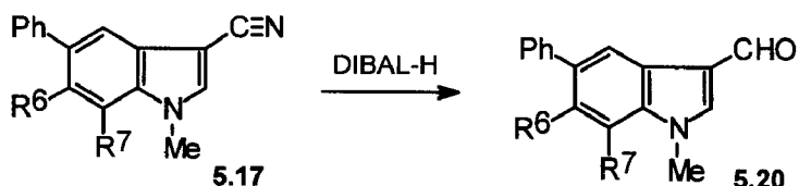
Scheme 5.7 : Conversion of 5.17 to 5.20 with DIBAL-H
