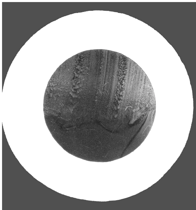
Figure 3. A picture of the cross-section of the polymer optical fiber. The surface has not been polished. The actual size is 0.95 mm for the core and 1.6 mm for the outer diameter of the fiber.
