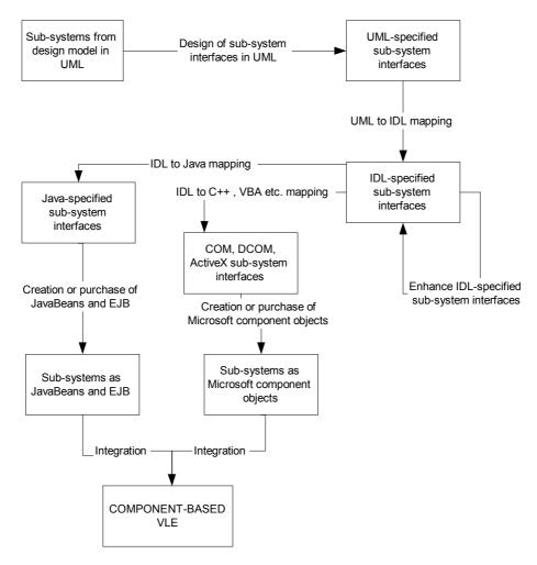
Fig. 3. Component development process
