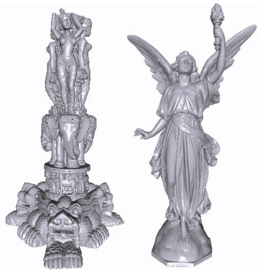
Fig. 6. Reconstruction of two large models ('Thai statue' and 'Lucy', 5 and 14 million samples, respectively) at octree level D = 11 .
