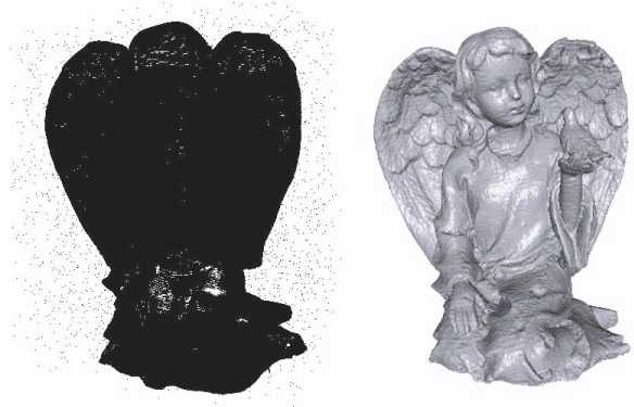
Fig. 8. Shot noise experiment. Left : noisy range data set with 2,008,414 samples and 4,000 outliers; right : reconstructed surface (CPU time: 168 seconds). Angel data set courtesy of the U.C. Berkeley Computer Animation and Modeling Group.
