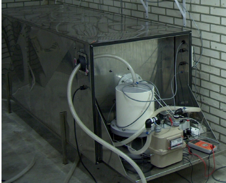
Fig. 2.6 A. ^{222}\text{Rn} detector (inlet at 60m).
