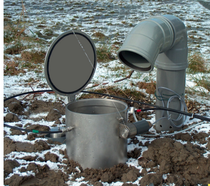
Fig. 2.6 B. ^{222}\text{Rn} soil chamber.
