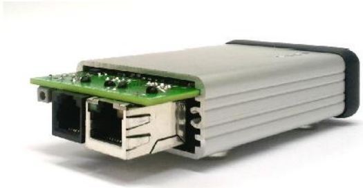
Figure 5: The Smart Meter gateway.
