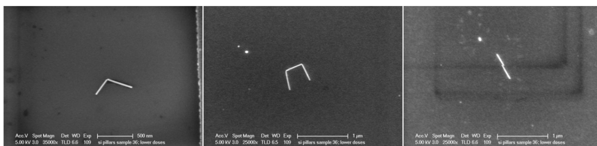
Fig. 17: Individual cases where two or three gold nanorods are linked via cysteine molecules.
