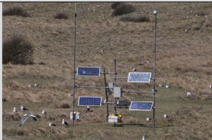
Ground station "Houston Control", 24 April 2010. In this version a radio antenna and receiver system (ARTS) were combined with the UvA BiTS GPS tracking base station. Solar panels and batteries provide the necessary power throughout the season. The onboard laptop computer could be remotely accessed through internet.
