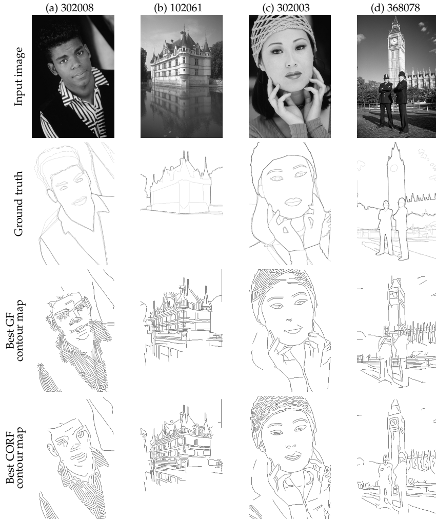
Figure 2.13: (First row) Images of natural objects from the Berkeley data set. (Second row) Ground truth illustrated as a superimposition of the collection of multiple contour maps drawn by different observers. Darker contours correspond to the agreement of multiple hand drawn contours. Optimal contour maps obtained by (third row) the GF and by (fourth row) the proposed CORF models, respectively.
