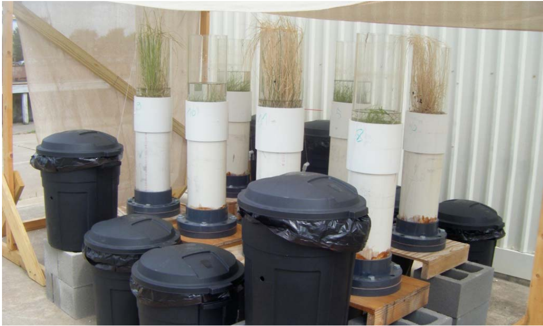
Figure 10 - Vegetated Test Columns during Pollutant Dosing
