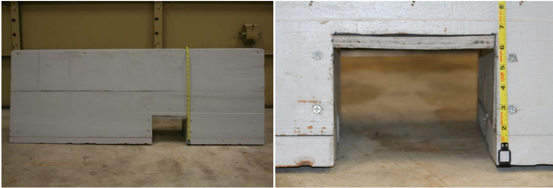
Figure 6.1 – Original MSSCB with no Clogging
