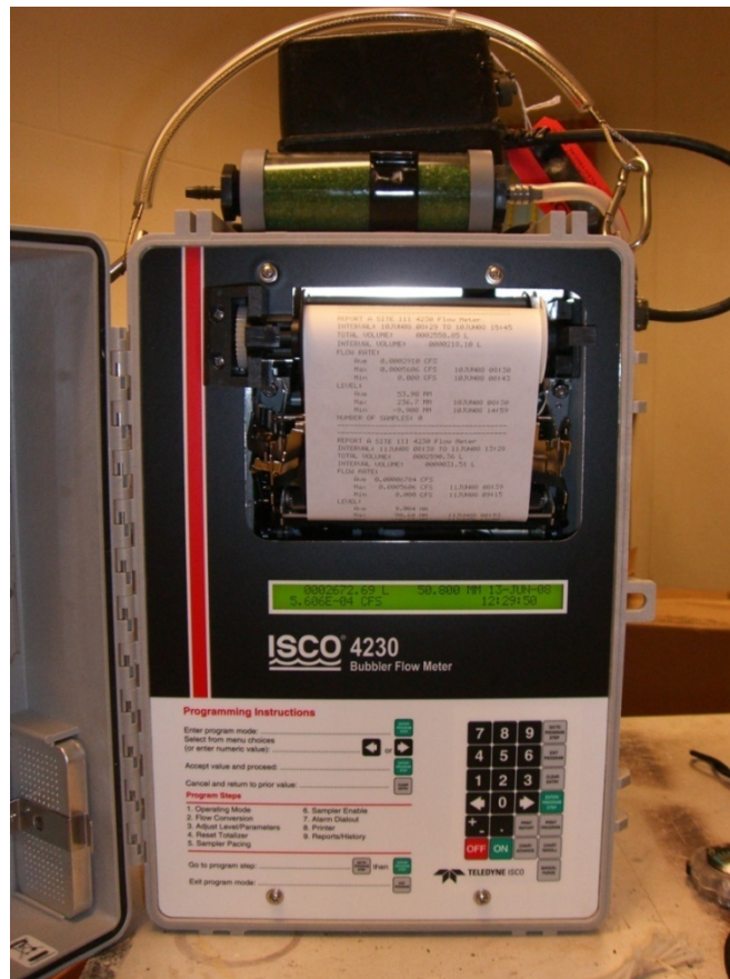
Figure 3.10 – ISCO bubbler used to measure standpipe head
