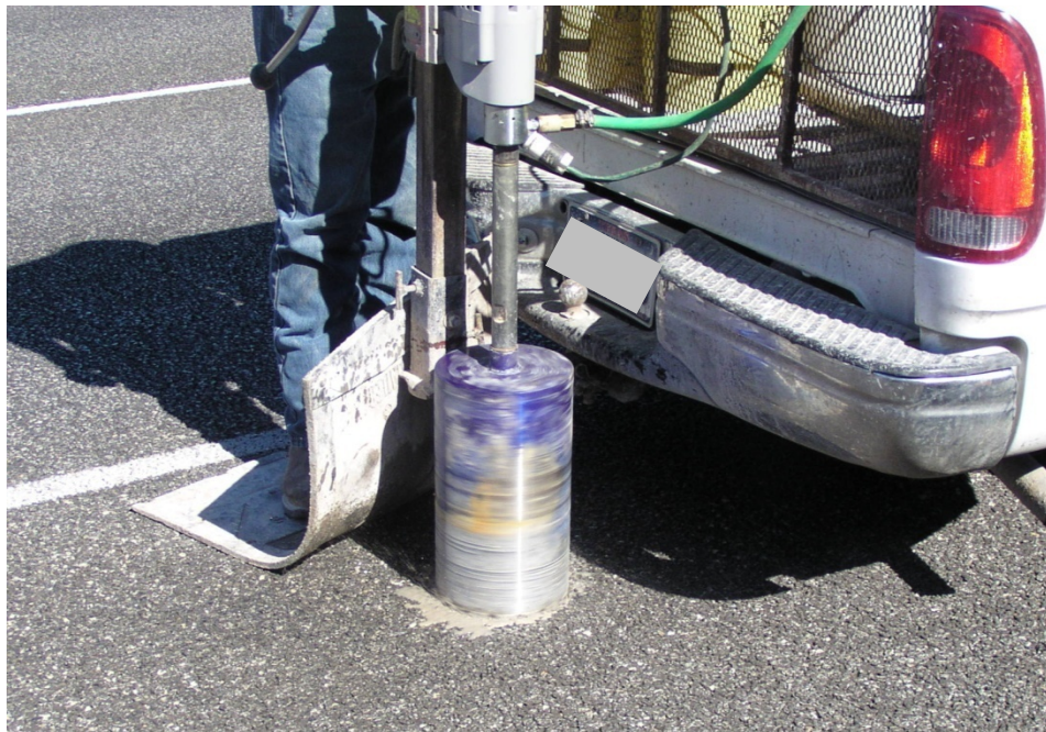
Figure 3.1 – Drill press used for core extraction
