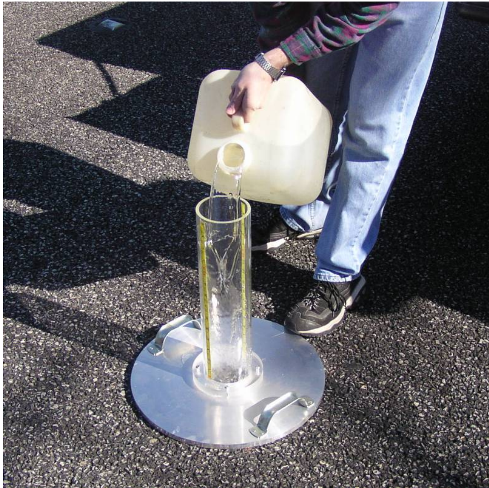
Figure 4.2 – CRWR field test apparatus
