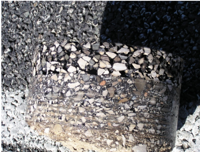
Figure 3.2 – Extracted PFC core with porous layer and impermeable base
