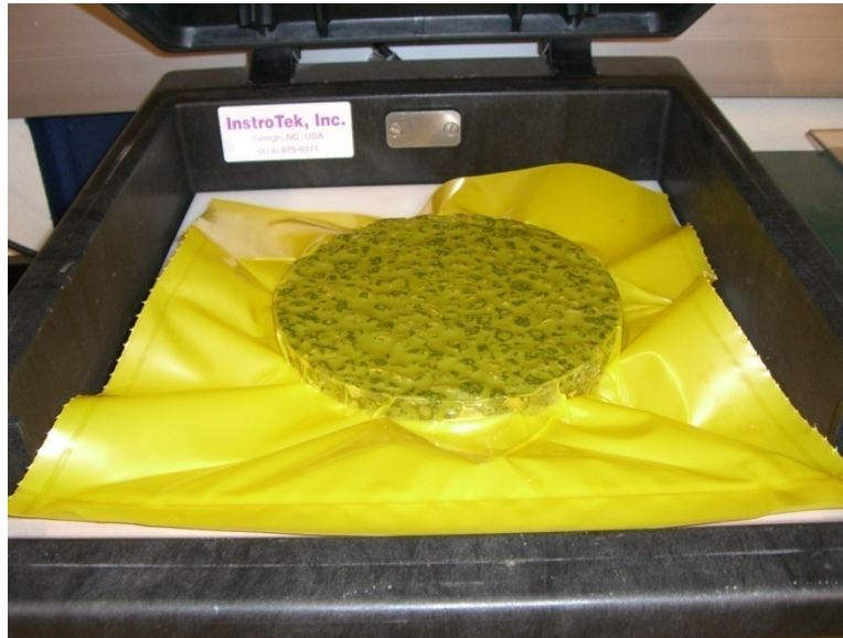
Figure 3.7 – PFC core vacuum sealed in plastic bag for porosity measurement
