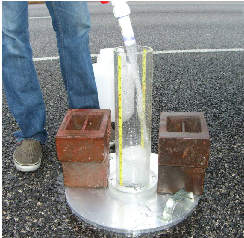
Figure 4.5 – Constant head field test
