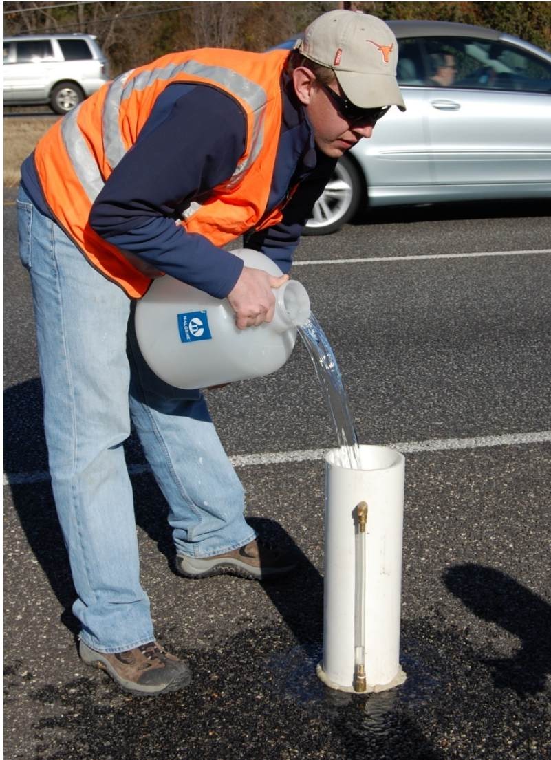
Figure 4.1 – Current TxDOT PFC drainage capacity test
