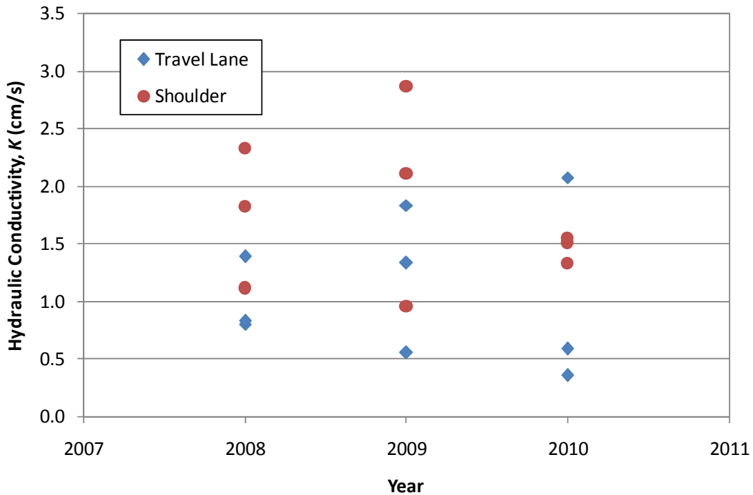
Figure 6.7 – Travel lane versus shoulder hydraulic conductivity data on Loop 360
