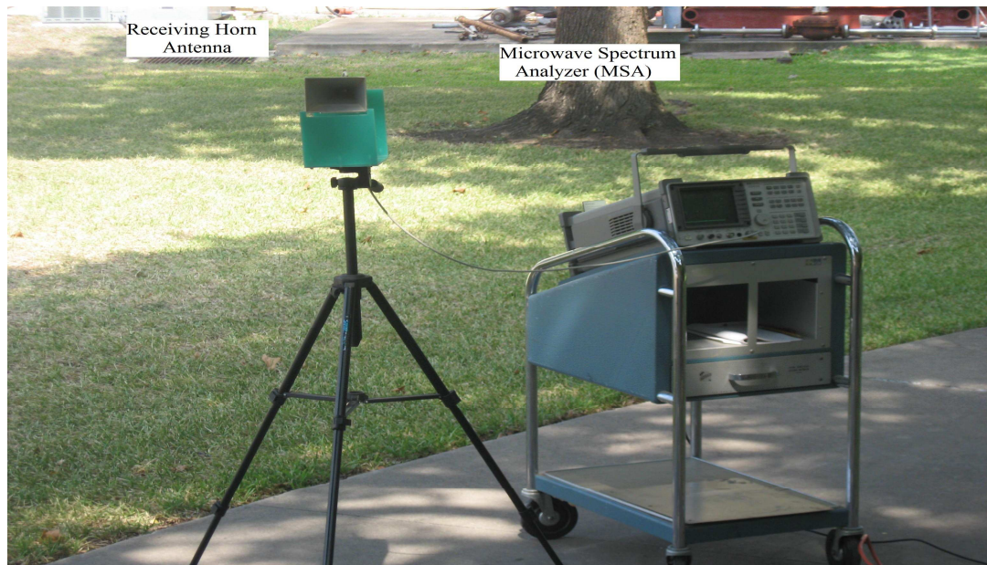
Fig. 4.2 Experimental setup of the PAA in transmitting mode (a) Overall setup along with an expanded view of the antenna array is shown. (b) The four TTD lines are shown. The inset shows the composition of each line. (c) The receiving horn antenna and the microwave spectrum analyzer are shown
