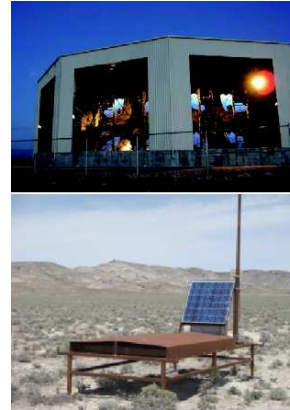
Figure 2: Top: Telescope array Fluorescence Detector (LR, BR) Bottom: Surface Detector deployed in the field.
