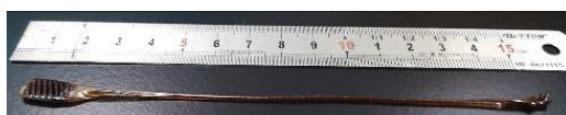
Figure S4. The recovered poly(TA-DIB-Fe) copolymer [Iron(III)-to-TA molar ratio of 1/100] after stressed.
