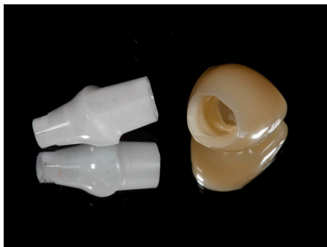
Fig. 2. Example of a debonding failure within a clinical study of a LU crown luted to a Zirdesign abutment. The design of the crown that was used in the present study matched a specimen that failed twice within one year of clinical service (Schepke et al., 2016).
