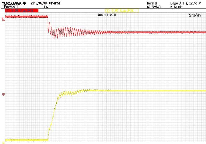
Fig. 15. System response to a step from P = 10 W to P = 300 W with the controlled shunt damper. Red curve (top) corresponds to the voltage x_2 (5 V/div) and yellow curve (bottom) corresponds to the current x_1 (5 A/div). Time scale is 2 ms/div.
