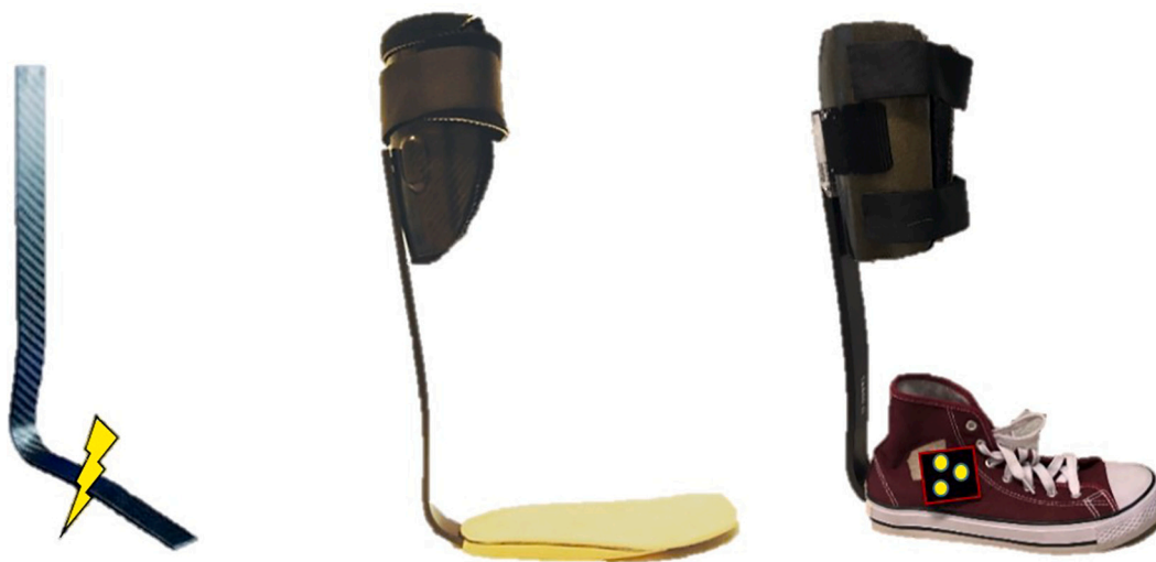
Fig. 1. Experimental AFO consisting of a carbon Ankle7 leafspring from which the foot part was shortened (left panel) and fixed to replaceable footplates with different stiffness levels (middle panel). The leafspring was connected through the back of the shoe to the footplate in a flexible sneaker. The cluster marker on the hindfoot is highlighted (right panel).
