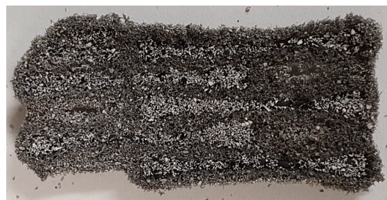
Fig. 9. Set of tensile test specimens of the type 1bb of dUHMWPE@silica with the addition of 1 wt% of nano silica and 0.25 wt% of CB built by PBF with the best practice parameters.
