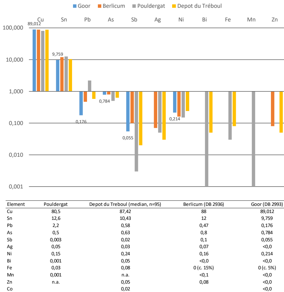
Figure 6. Bar-chart (top, labels for the Goor spearhead added) and table (bottom) for the Tréboul alloys analysed (Pouldergat: Briard & Onnée 1971, 31, Tréboul hoard: Cecile le Carlier de Veslud, pers. comm. March 2021, Berlicum: Van Os in Ruijters 2020, appendix 7, Goor: this study).
