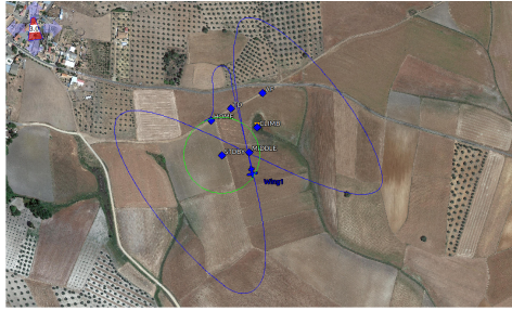
Figure 9.6: The screenshot of the ground control station corresponding to Fig. 9.5. The green circle is the stand-by trajectory before the aircraft starts following the Lissajous curve. The blue line is the 2D trajectory of the aircraft. In particular, the aircraft passes by the middle waypoint corresponding to the highest point of the desired path.
