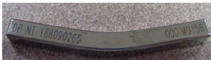
Figure 1. Square, anatomically shaped NiTi alloy Spinal Rod.
