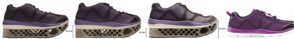
Fig. 3. From left to right: Experimental shoes R16, R18.5, R21 and the control shoe. The holes in the internal structure of the experimental outsoles are for weight reduction. All experimental outsoles had a thickness of 35 mm and a toe spring of 20 mm.
