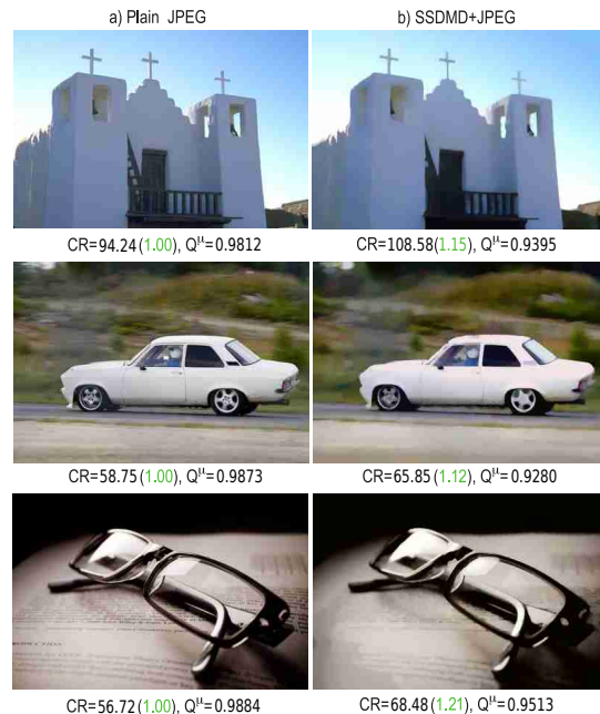
Figure 8: Comparison of JPEG (a) with the SSDMD method applied as preprocessor to JPEG (b) for three images. Green values show CR gains as compared to JPEG.
