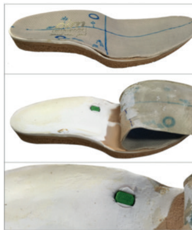
Fig. 1. Custom-made inlay with built-in sensor.
